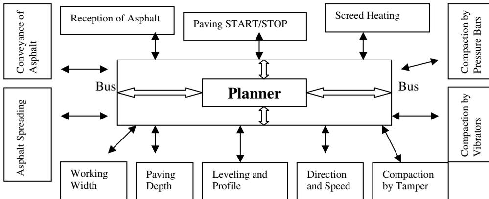
**Figure 4: Block Diagram of Functional Modules for the Automated Road Paver**
